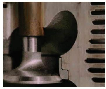
Figure 2–Lycoming "morning sickness" is caused by buildup of exhaust deposits on the exhaust valve stem and inside the exhaust valve guide. The cure is to clean the valve stem and ream the valve guide, something that can be done without removing the cylinder.
