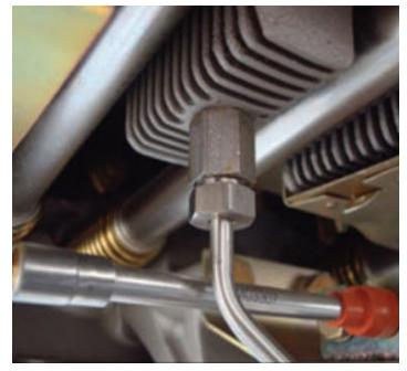
Figure 3—The CHT probes in Cirrus aircraft are notorious for failing and providing erroneous CHT data.
