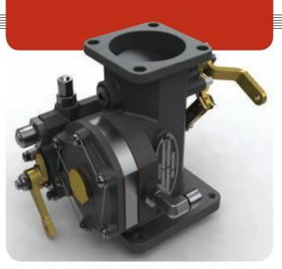
Figure 1–Two local mechanics decided that the RSA fuel servo was the culprit .
